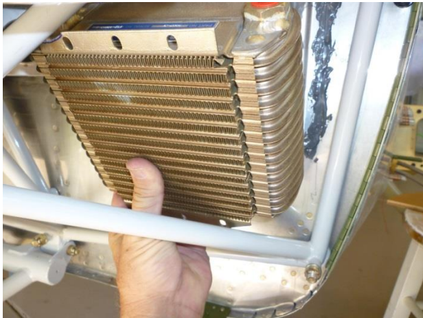
Figure 5: Shows the lower, forward, outboard corner of the oil cooler modified to clear the engine mount tube. Use only tin snips to make this cut
