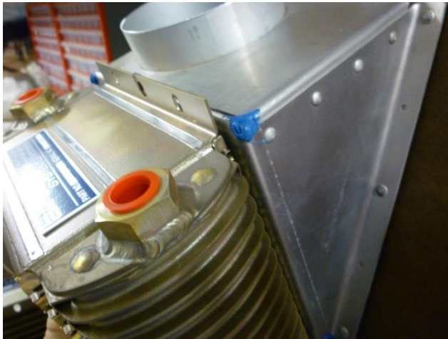
Figure 1: Shows the 2007X in position on the stock air box. Note the 2007X mounting flange extends above the stock air-box
