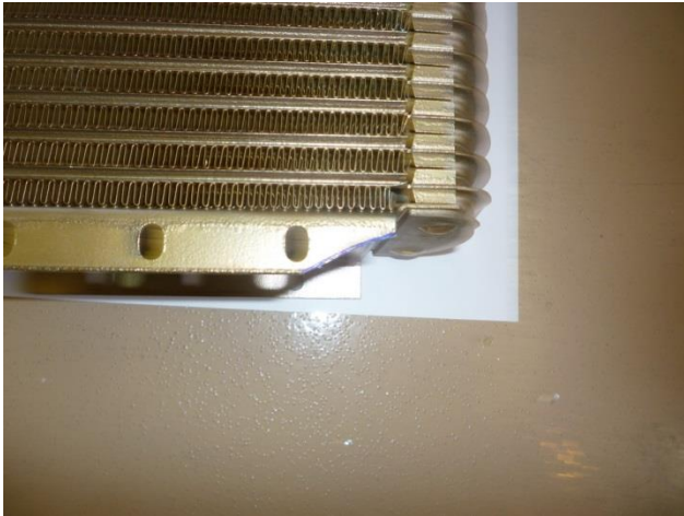
Figure 5: Shows the lower, forward, outboard corner of the oil cooler modified to clear the engine mount tube. Use only tin snips to make this cut
